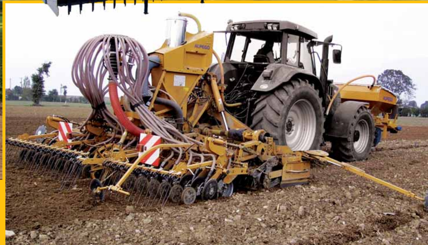
COMBINAZIONE AS3 CON ERPICE DX MINIMA LAVORAZIONE PER SEMINA SU SODO • A COMBINATION OF THE AS3 WITH A DX HARROW MINIMUM STRESS WHEN WORKING ON FIRM GROUND • KOMBINATION AS3 MIT ERGGE DX MINIMALE BEARBEITUNG FÜR BODENAUSSAAT
